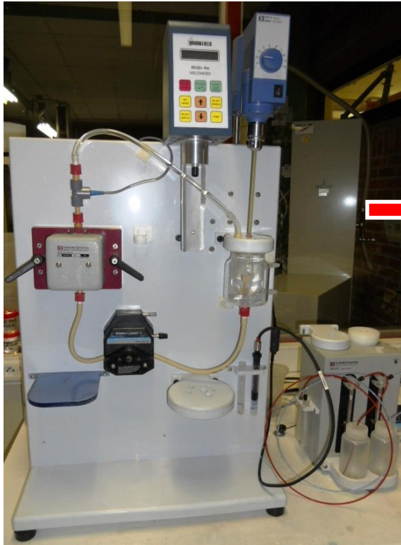
\zeta potential measurement - adjustment (acoustic method)
