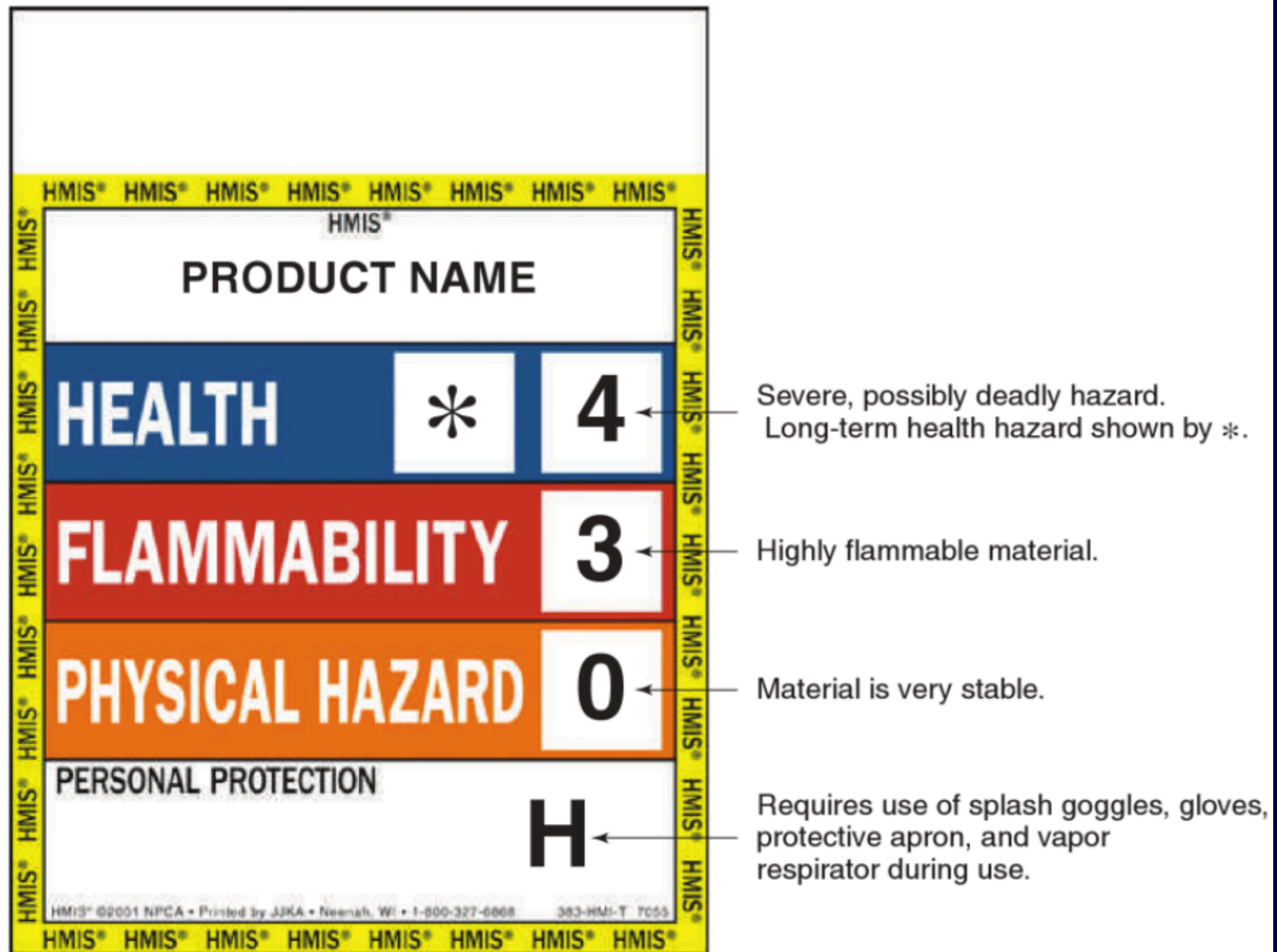
FIGURE 2.1.22 Explanation of two sample HMIS hazard labels.
