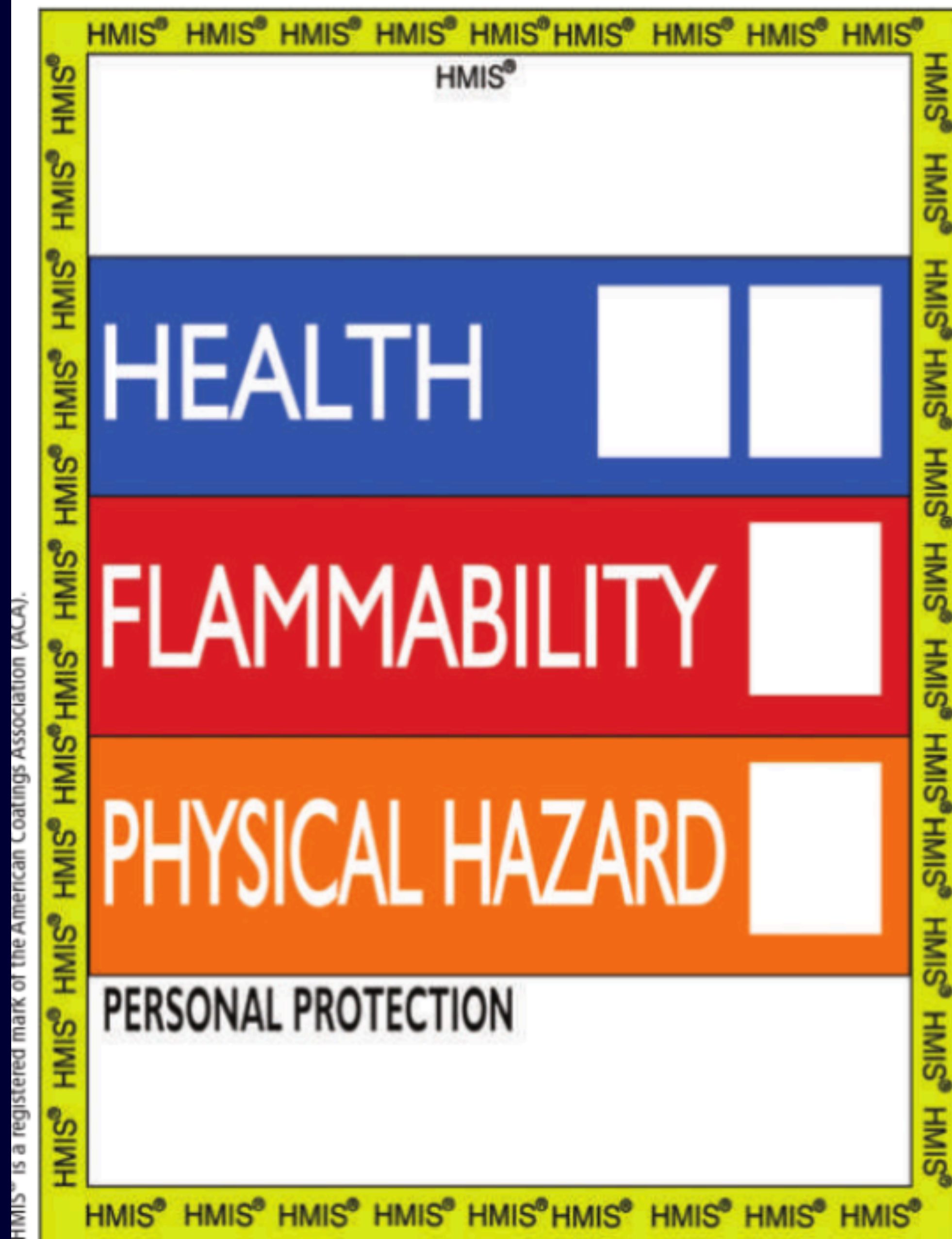
FIGURE 2.1.20 The HMIS III hazard label.
