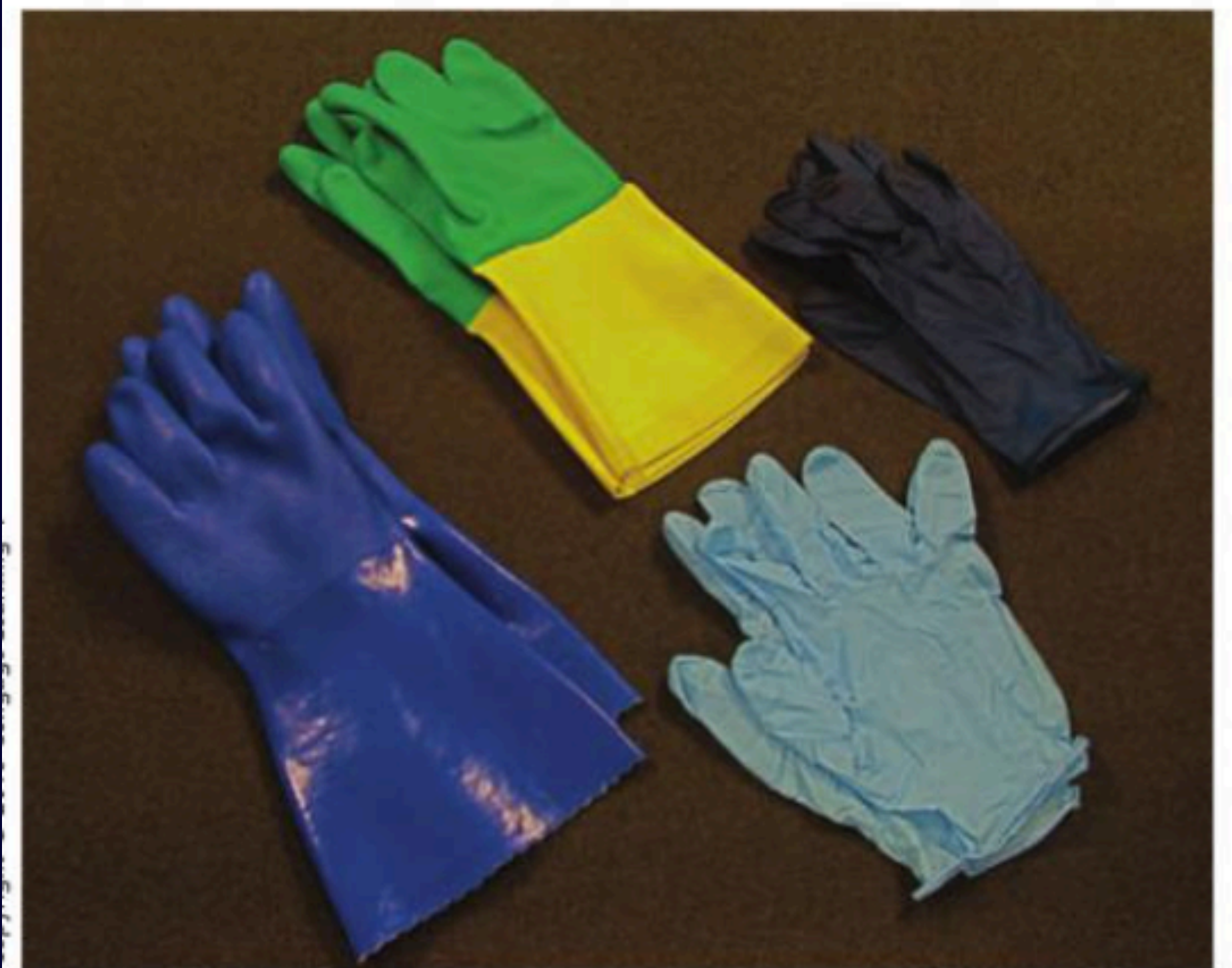
FIGURE 2.1.8 Different gloves are available for different uses. Note the different lengths. When handling chemicals, always follow the chemical manufacturer’s recommendation for the proper type of glove.
