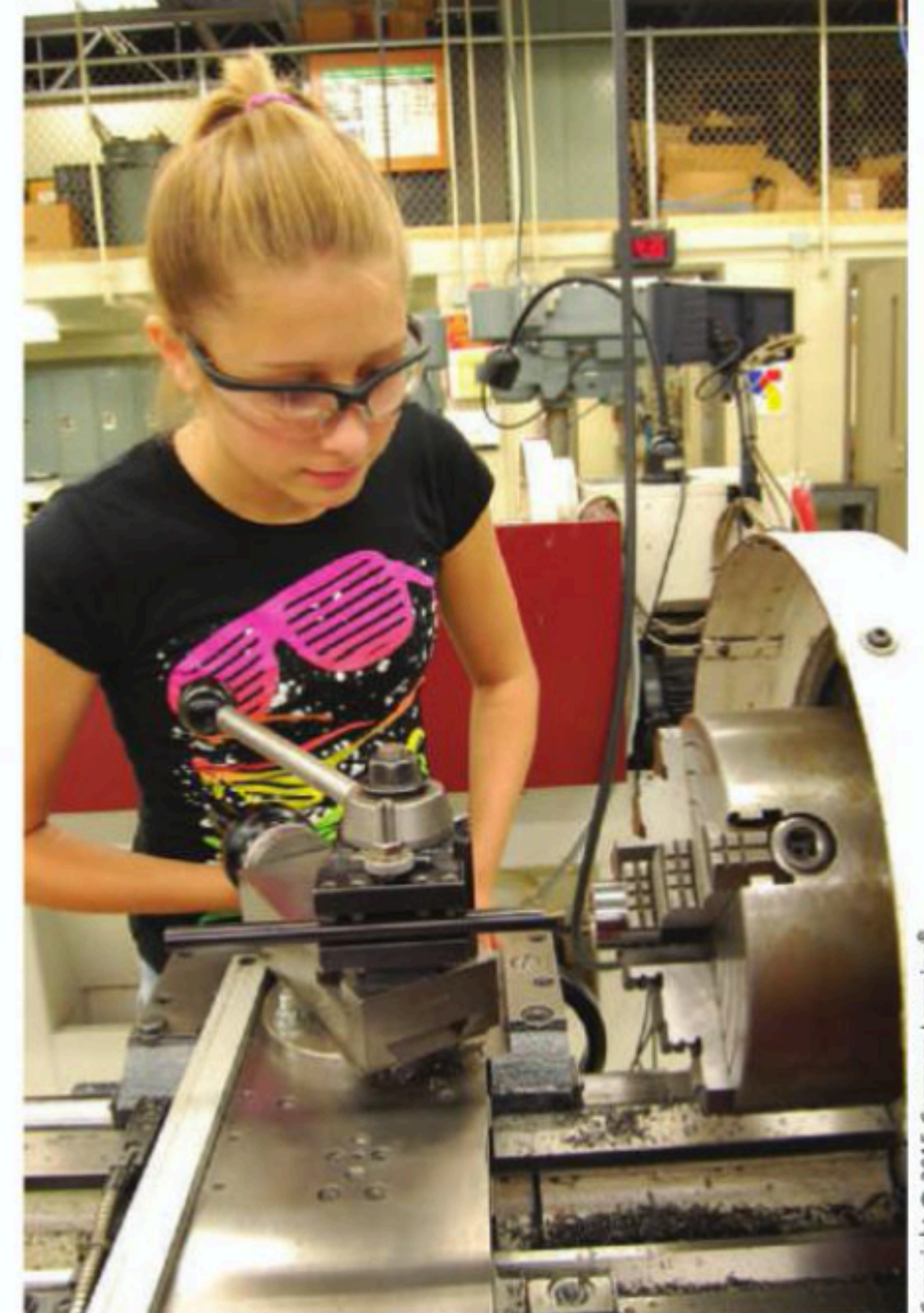
FIGURE 2.1.2 Long hair should be secured safely in a machining environment.
