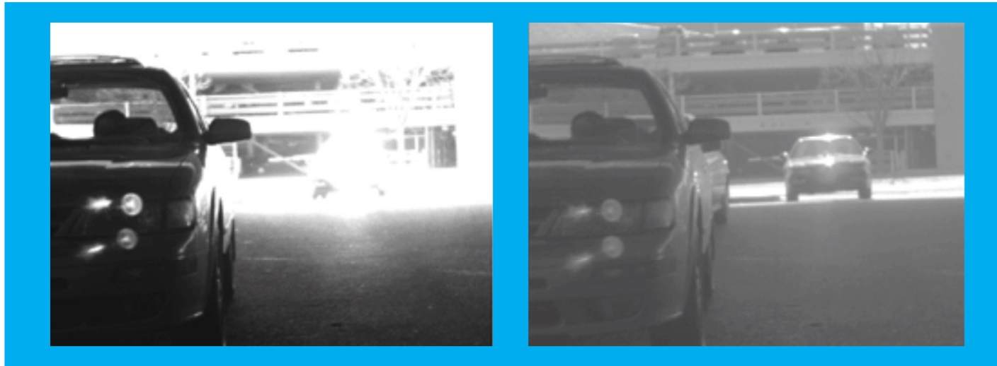
Figure 2. Images captured without (left) and with (right) Wide Dynamic Range
